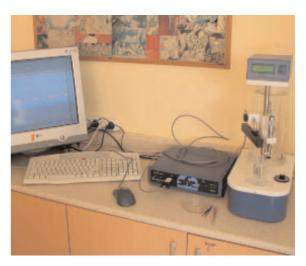
**Figure 2.** Muscle contractions were recorded to an IBMcompatible PC using a force displacement transducer (SS12LA, Biopac systems Inc., Santa Barbara, CA, USA) at 200 Hz sample rate to which the upper wire was connected. A Biopac MP35 (data acquisition system Biopac systems Inc., Santa Barbara, CA, USA) was used for the recordings and stimulations (Tasman/2000, Cehreli 2002).
